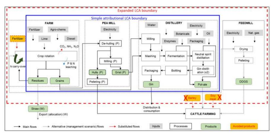
Figure 4. Processes considered within system boundaries for gin production from peas and wheat, based on simple attributional LCA (energy allocation) and system expansion
