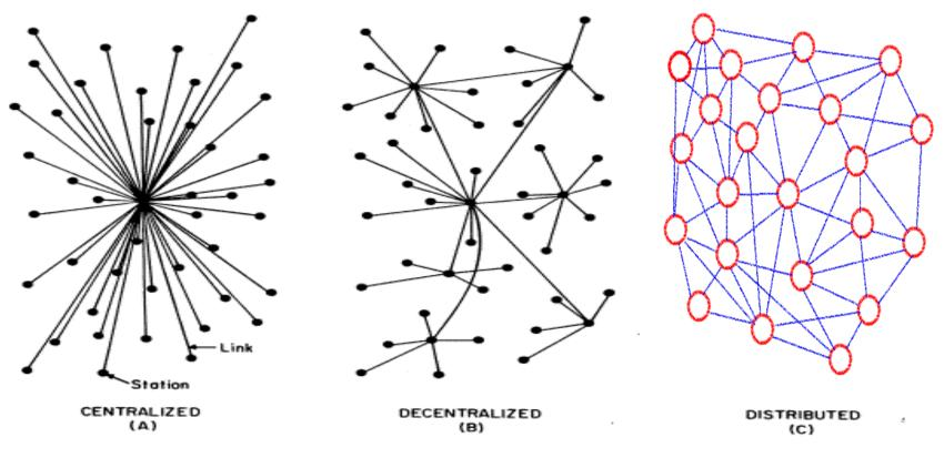
FIG. I - Centralized, Decentralized and Distributed Networks
