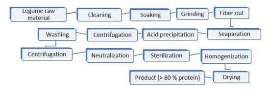
Figure 5. Processing steps to produce protein isolate from legumes.
