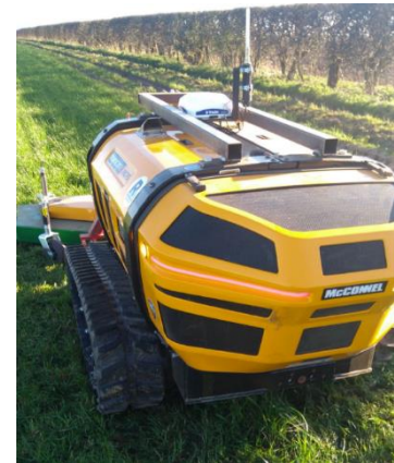
Figure 19. The autonomous prime mover prototype (TRL5) developed by Third party sub-contractor Manterra Ltd.
